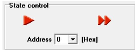
**Control field** It is used to select the address, start and reset the software of the unit IVM. The selected address must correspond to the position of the switch for selecting the address, which is located on the CAN BUS card of the corresponding unit.
