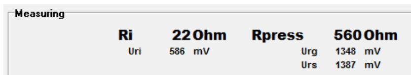
**Measuring field** This field shows the current measured values Ri (valve coil resistance for quick closing of the slide valve) and Rpress (pressure switch link resistance). (The values Uri, Urg, Urs are indicative only. These are the values of internal variables necessary for the calculation of resistance values)
