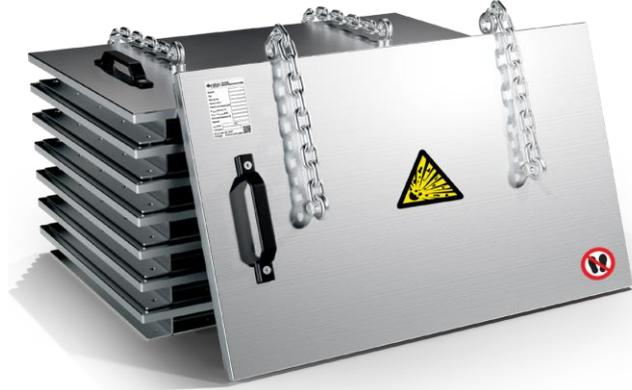
Under the designed operating conditions, the inner space of protected equipment of the ExDoor is sealed off. The vent panel on the frame bursts during an explosion, causing the vent path to open up.
