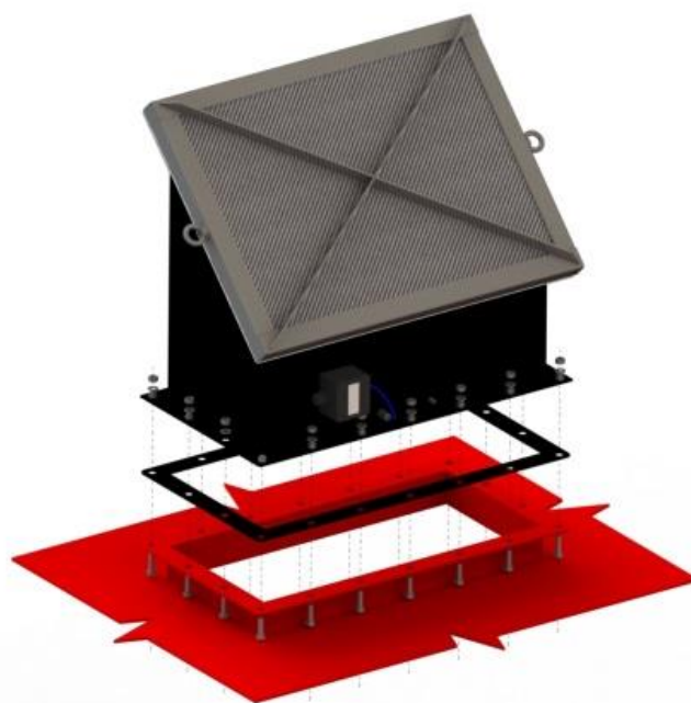
The exploded view of the flat FLEX (1 – FLEX, 2 – flange gasket, 3 – bolting materials, 4 – protected technology)
